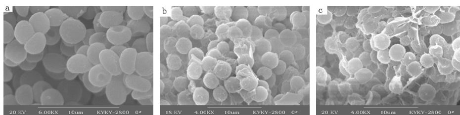
Figure 4 SEM pictures of sheep blood cell after exposure to membranes for 4.0 h. (a) control; (b) exposure to modified chitosan film; (c) exposure to chitosan film
